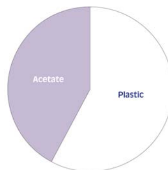
Fig 5: Estimate of Acetate / PVC-Polyester ratio based on a sample of 300 tapes, acetate tested translucent to light
